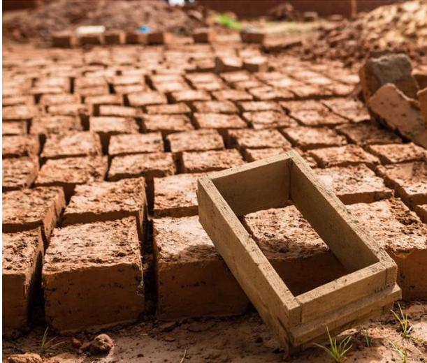
The bricks are dried in the sun, then they are stacked up and moved into ovens called “kilns” where the fire hardens the bricks, and finally the hot bricks are removed from the kiln to cool.
